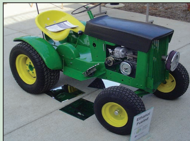
Figure 15. Garden Tractor Modified to Run on Ethanol by Students at Saginaw Valley State University
